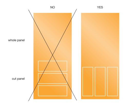
The cutting scheme should always be made considering that the longer side of the cut piece should always be parallel to the long side of the entire panel. This in order to minimize the dimensional variation of the panels, which is almost double on the short side of the panel, compared to the long side.
