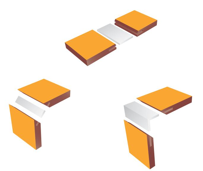
Restrained joint with aluminum profiles for mobile walls
