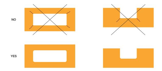
The holes and the internal corners should never present sharp corners, which could cause cracking, but should always be rounded with the maximum radius possible
